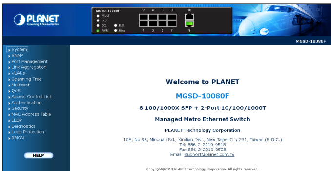
Figure 7-3: Web Main Screen of the Managed Switch
