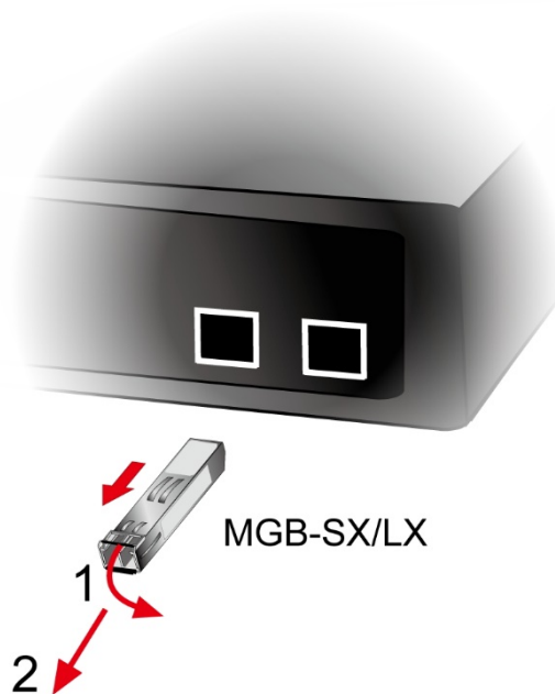
Figure 2-2-5: How to Pull Out the SFP/SFP+ Transceiver
