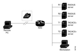
Figure 6-1 Typical AAA Network Configuration
