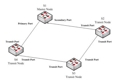
Figure 1.1 EAPS Ethernet ring
