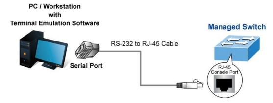
Figure 3-1 Out-of-Band Management Configuration Environment
