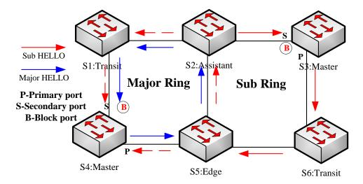
Figure 5: Intersection of the major ring and the sub ring
