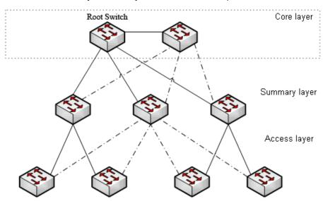
Figure 1.2 Switching network topology
