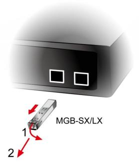
Figure 2-6: How to Pull Out the SFP/SFP+Transceiver
