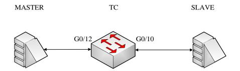
**MASTER** here stands for the master clock, which is a L2 PTP device. **SLAVE** here stands for the master clock, which is a L3 PTP device. TC stands for a switch that supports transparent clock. The master clock connects port g0/12 of the switch, while the slave clock connects port g0/10 of the switch. MASTER, TC and SLAVE are all working in P2P mode. Ports g0/10 and G0/12 belong to VLAN1.
