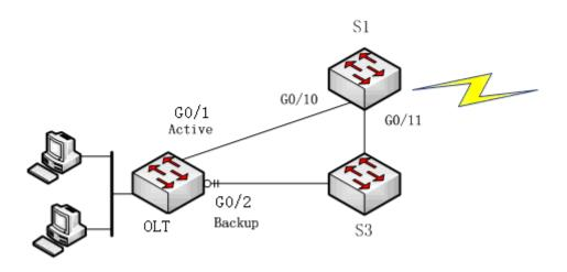
Figure 2: FlexLinkLite configuration example
