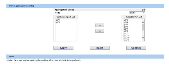
Figure 9: Setting the member port of the aggregation group
