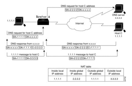
Figure 43-3 Network Condition Where NAT Translates Overlapping Addresses
