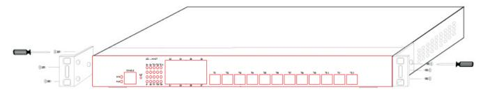
Figure 2-4 Attach brackets to the Managed Switch.
