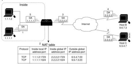
Figure 43-2 NAT Operation During the Reloading of Inside Global Address
