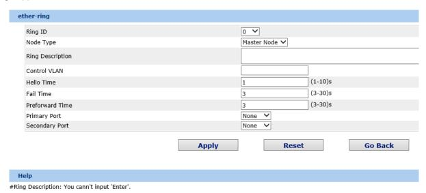
Figure 20: EAPS ring configuration
