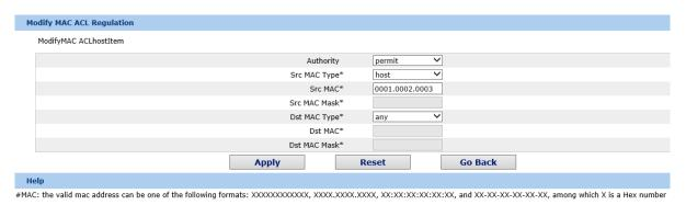
Figure 7: Setting the Rules of the MAC Access Control List
