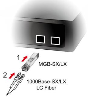
Figure 2-5 Plug in the SFP transceiver
