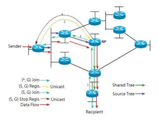
Figure 5-1 Join-in mechanism of PIM-SM
