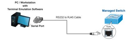
Figure 4-1: Managed Metro Switch Console Connectivity
