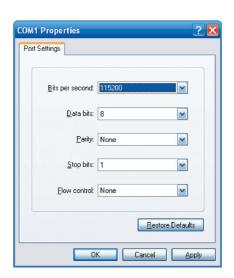
Figure 4-2: COM Port Configuration
