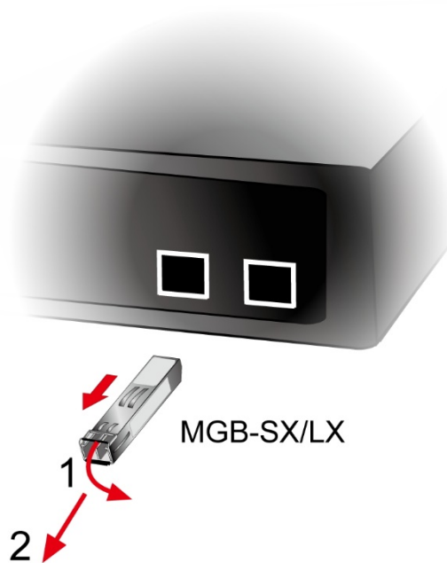
Figure 2-2-5: How to Pull Out the SFP/SFP+ Transceiver
