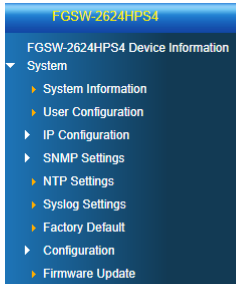
Figure 4-2-1: Managed PoE+ Switch System Web Page
