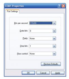
Figure 3-2: COM Port Configuration
